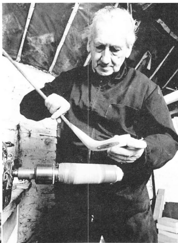
5. The head and shaft spliced together, the joint is cleaned up on a rotary sander.
