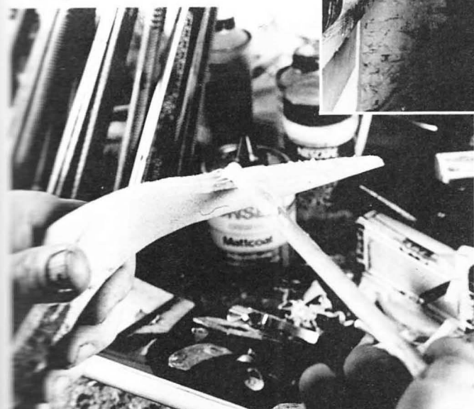
4. Neck and shaft are joined by a long splice. Here the neck half is being glued for assembly. The splice will be further strengthened with twine whipping.
