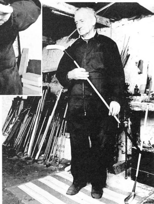
6. Jointed, and with lead and ram's horn in place, the club's 'whip' and 'loft' are gauged. Its whip can be increased by careful sanding. It then gets a final polish, whipping on the splice, a leather grip, its maker's name on its head, and is stained and varnished.
